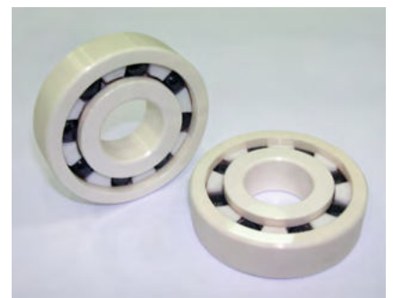
Full Ceramic Bearing Zirconia inner ring, outer ring and rolling element. Silicon nitride ball
